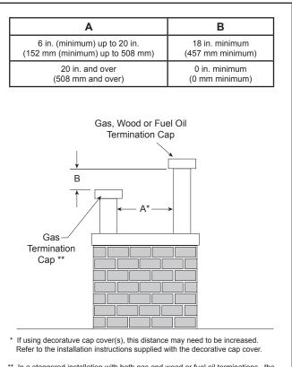
\*\* In a staggered installation with both gas and wood or fuel oil terminations, the wood or fuel oil termination cap must be higher than the gas termination cap.
